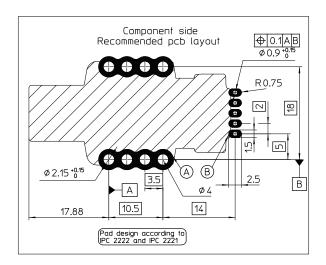
(Layout example with 4 jumpers in parallel)
