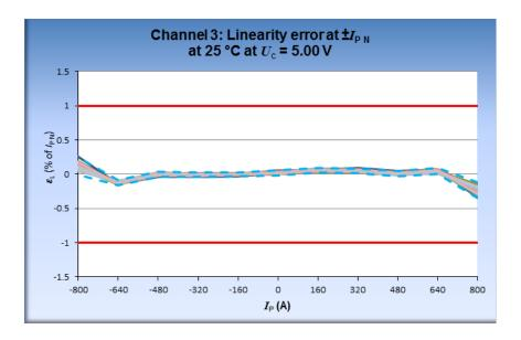
Curve extract from PV test. Dotted line represents the  $3\sigma$  limit
