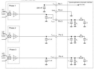
$C_{L}$ < 2.2 nF EMC protection (optional) RC Low pass filter (optional)
