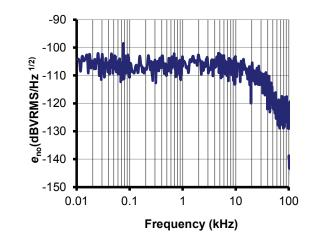
Figure 12: Typical noise voltage spectral density  $e_{no}$ with  $R_{\rm M}$  = 50  $\Omega$
