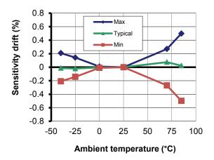
Figure 5: Sensitivity thermal drift
