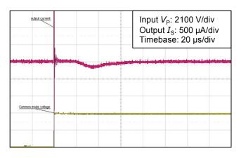
Figure 11: Detail of typical common mode perturbation (4200 V step with 6 kV/ $\mu$ s,  $R_{\rm M}$  = 100  $\Omega$ )
