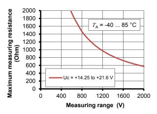
Figure 1: Maximum measuring resistance
