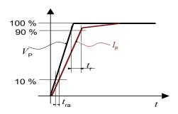
Figure 15: response time  $t_r$  and reaction time  $t_{ra}$
