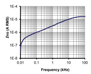
Typical total output RMS noise current Figure 13: with  $R_{\rm M}$  = 50  $\Omega$
