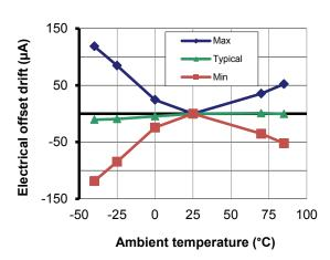
Figure 3: Electrical offset thermal drift
