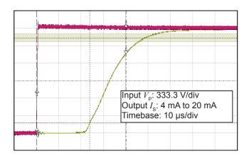
Figure 10: Typical step response (0 to  $V_{\rm P\,N}$ )
