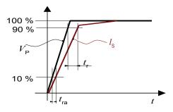
Figure 15: response time  $t_r$  and reaction time  $t_r$
