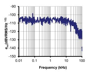
Figure 11: Typical noise voltage density  $e_{no}$  with  $R_{\rm M}$ = 50  $\Omega$
