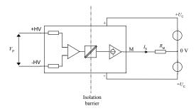
Figure 14: standard characterization schematics for current output transducers ( $R_{\rm M}$  = 50  $\Omega$  unless otherwise noted)
