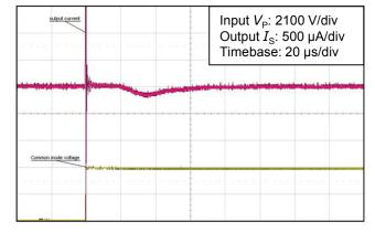
Figure 5: Typical step response (0 to 1000V)
