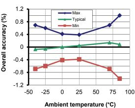
Figure 2: Electrical offset thermal drift
