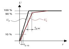
Figure 19: Delay time  $t_{\mathrm{D}\,90}$  @ 90 and delay time  $t_{\mathrm{D}\,10}$  @ 10
