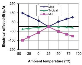
Figure 3: Electrical offset thermal drift
