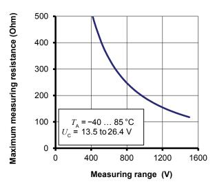
Figure 1: Maximum measuring resistance
