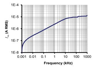
Figure 16: Typical total output RMS noise current with  $R_{\rm M}$  = 50  $\Omega$
