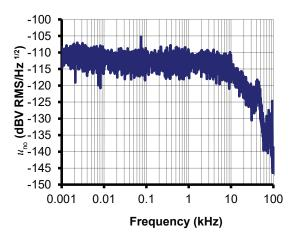
Figure 15: Typical noise voltage spectral density  $u_{\rm no}$  with  $R_{\rm M}$  = 50  $\Omega$
