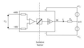
Figure 18: Standard characterization schematics for current output transducers ( $R_{\rm M}$  = 50  $\Omega$  unless otherwise noted)
