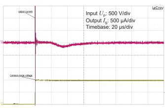
Figure 14: Detail of typical common mode perturbation (1000 V step with 6 kV/ $\mu$ s,  $R_{\rm M}$  = 100  $\Omega$ )
