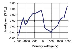
Figure 17: Typical linearity error at 25 °C
