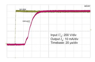
Figure 6: Typical step response (0 to 1000 V)
