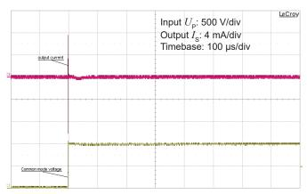
Figure 13: Typical common mode perturbation (1000 V step with 6 kV/ $\mu$ s  $R_{\rm M}$  = 100  $\Omega$ )
