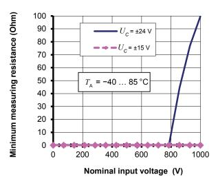
Figure 2: Minimum measuring resistance The derating @  $\pm 24$  V is only applicable for  $T_{\rm A}$  = 80 ... 85 °C For  $T_{\rm A}$  under 80 °C, the minimum measuring resistance is 0  $\Omega$  whatever  $U_{\rm C}$
