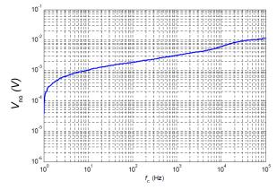
Figure 3: Output noise voltage, cumulated rms
