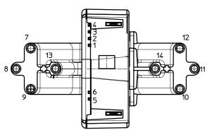
The four integrated primary conductors have a diameter of 2.5 mm. The three conductors 7-12, 8-11 and 9-10 could be used as the lines in a three phase system; the conductor 13-14 could be used either as the neutral in a three phase system or as a test current conductor.
