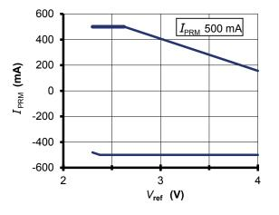
Upper limit:  $I_p$ =500 mA $(V_{ref} = 2.3 \dots 2.625 \text{ V})$ Upper limit:  $I_p$ =-250 \*  $V_{ref}$  + 1156.25 $(V_{ref} = 2.625 \dots 4 \text{ V})$ Lower limit:  $I_p$ =-250 \*  $V_{ref}$  + 93.75 $(V_{ref} = 2.3 \dots 2.375 \text{ V})$ Lower limit:  $I_p$ =-500 mA $(V_{ref} = 2.375 \dots 4 \text{ V})$
